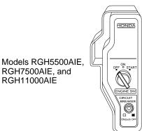
Figure 29 - Engine Switch In OFF Position
